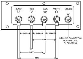
Figure 23. Output Terminal Lugs 3Ø 240/139V Connections
